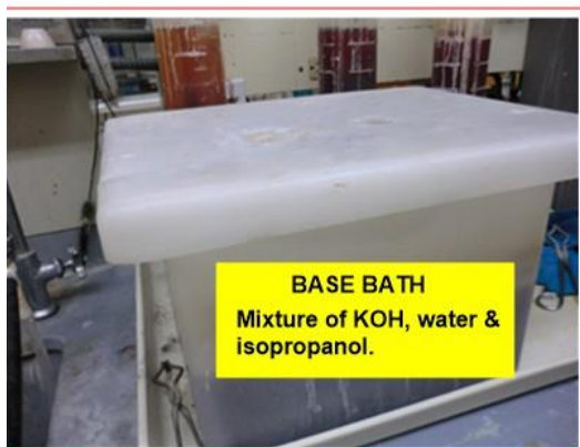
Fig. 1: A Base Bath Near a Sink
