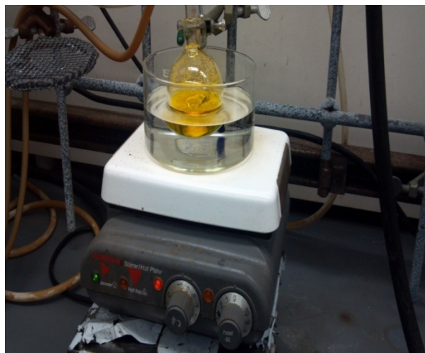
Fig. 1: Use of hot plate for heating and stirring the reaction
