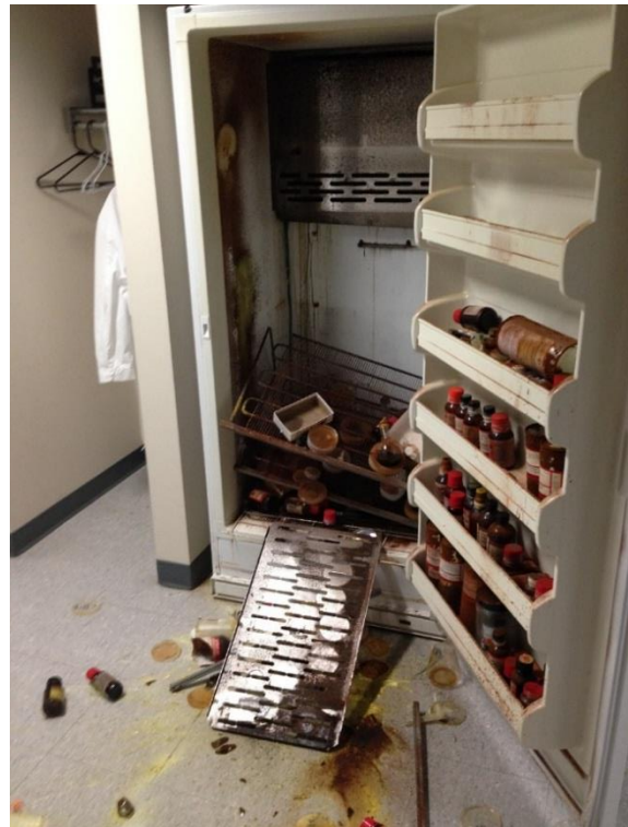
Figure 1: Corroded refrigerator causes chemical spill
