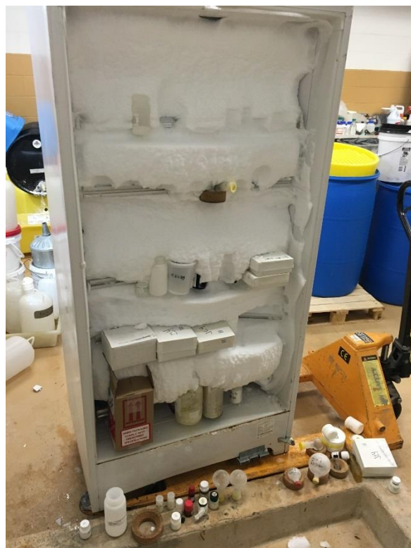
Figure 2: Abandoned chemical freezer frozen over
